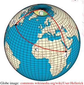
$\cos^{-1}(\cos(48^\circ)\cos(81^\circ) + \sin(48^\circ)\sin(81^\circ)\cos(110^\circ))$ which is about  $98^{\circ} = 98 \times 60$  nautical miles (1 nautical mile = 1 minute of great circle arc), or about 10900km.
